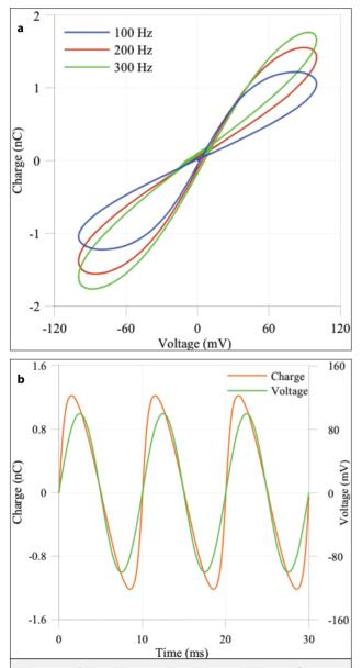
Figure 2. a,b. Simulation results under sinusoidal inputs for memcapacitor. a) Voltage-current relationship with various frequencies. b) Charge and input voltage of memcapacitor
