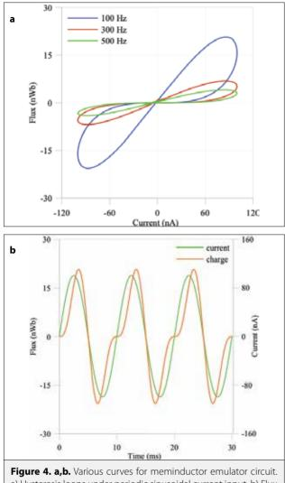
a) Hysteresis loops under periodic sinusoidal current input. b) Flux and input current of meminductor
