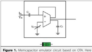
Figure 1. Memcapacitor emulator circuit based on OTA. Here C1=1nF, C2=1pF, gm=3mS
