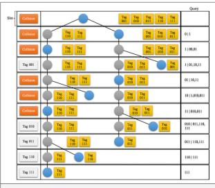
Figure 8. Tag identification using the query tree protocol
