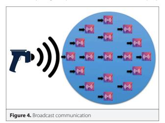
region of a single reader. There are two main communication protocols as broadcast and multiple access in such a system. Broadcast communication is applied to transmit data from the reader to the tags. The data sent by the reader is taken simultaneously by all the tags in the query area of the reader (Figure 4). This comminication protocol can be imagened as the simultaneous reception of a news program transmitted by a radio station to the hundreds of radio receivers [1, 11].
