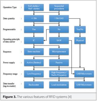
**Operation frequency:** When selecting a frequency for an RFID system, the characteristic of several available frequency ranges must be taken into account. The availability of applicable frequencies and frequency bands in the operating area of the system has a significant impact on the system parameters [1, 4].
