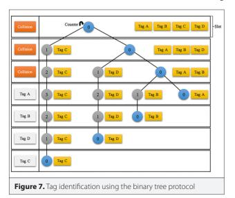
the number of tag sets that the reader should recognize. Otherwise, the reader decreases the counter value by 1. When the reader's counter value is less than 0 (counter value<0), the reader terminates the frame [10, 13, 17].
