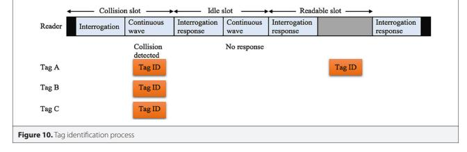
system. Based on the number of tag ID transmissions in a query period, the tag reading process is divided into three parts on the reader side:
