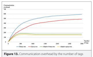
increases, the performance of query tree-based protocols deteriorates. Query tree-based protocols, as compared to binary tree-based protocols, have long tag identification delay and high tag communication overhead because the reader sends all interrogations leading to collisions in every frame and the number of idle cycles increases [1, 10, 13].
