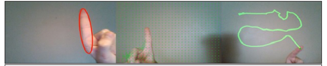
Figure 4. Tracking Algorithms as CamShift, Dense Optical Flow and Sparse Optical Flow
