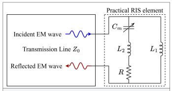
Fig. 1. The equivalent circuit of a practical RIS element.
