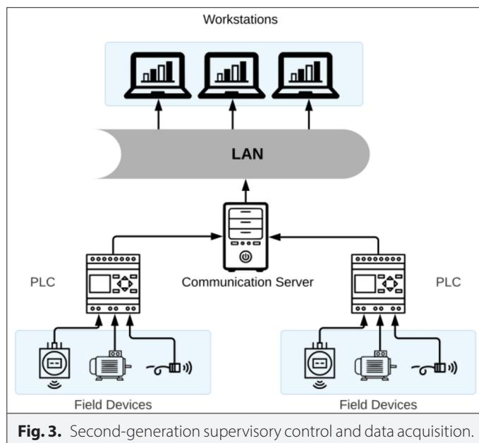
**Fig. 3.** Second-generation supervisory control and data acquisition.
