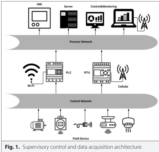
**Fig. 1.** Supervisory control and data acquisition architecture.
