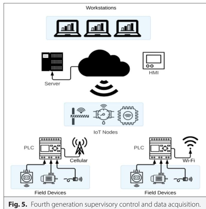
**Fig. 5.** Fourth generation supervisory control and data acquisition.
