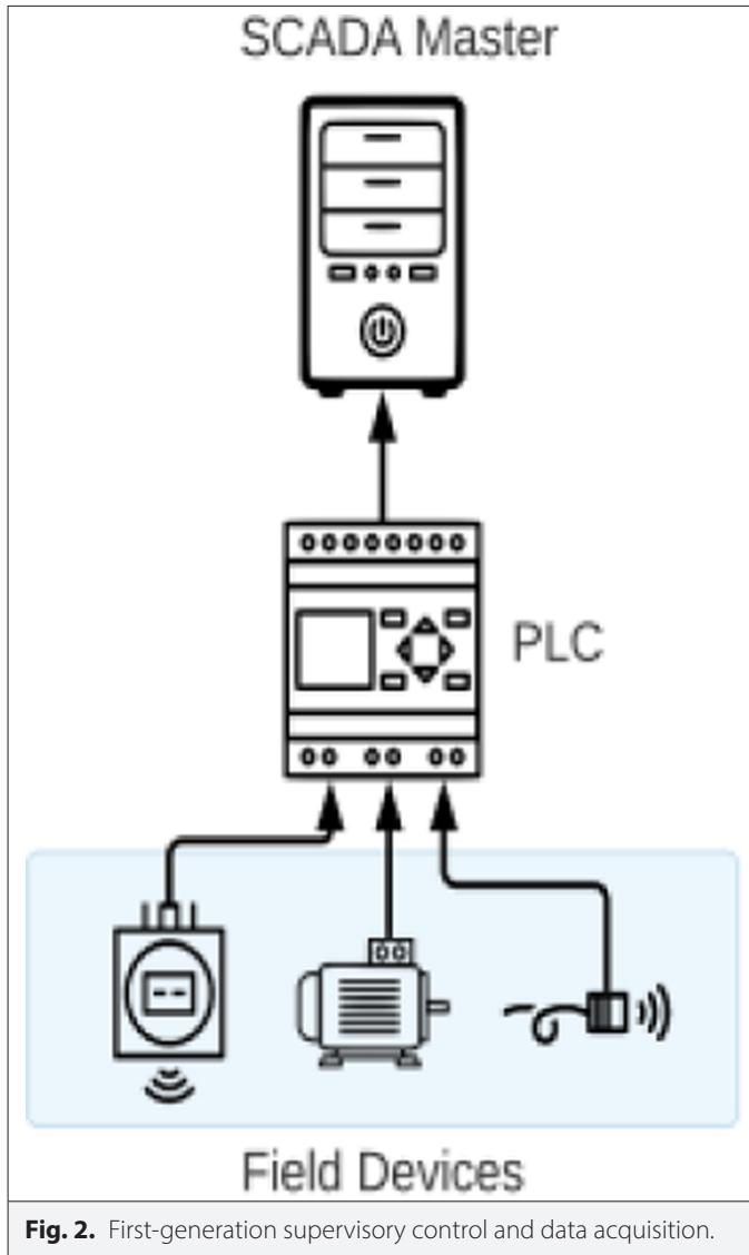
**Fig. 2.** First-generation supervisory control and data acquisition.
