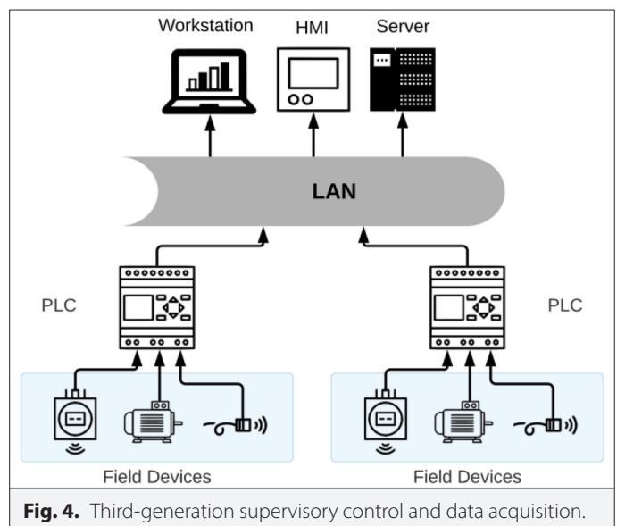
**Fig. 4.** Third-generation supervisory control and data acquisition.
