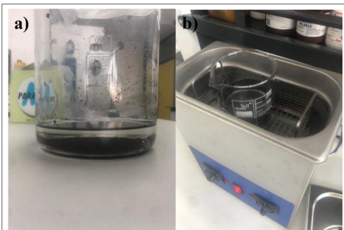
Fig. 3. Graphite oxide that settles to the bottom because of resting (a), the ultrasonic bathing phase of graphite oxide (b) [32].
