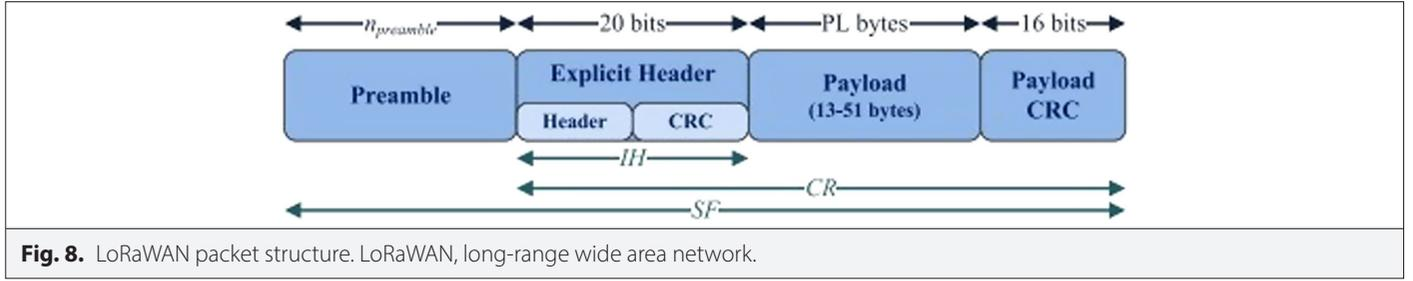
**Fig. 8.** LoRaWAN packet structure. LoRaWAN, long-range wide area network.
