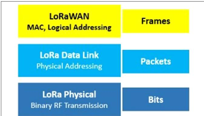
Fig. 2. LoRaWAN layered architecture. LoRaWAN, long-range wide area network.
