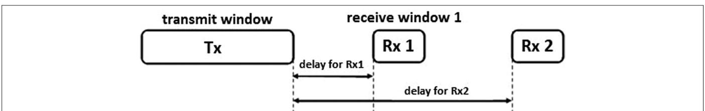
Fig. 3. Transmit and receive windows for class A device.
