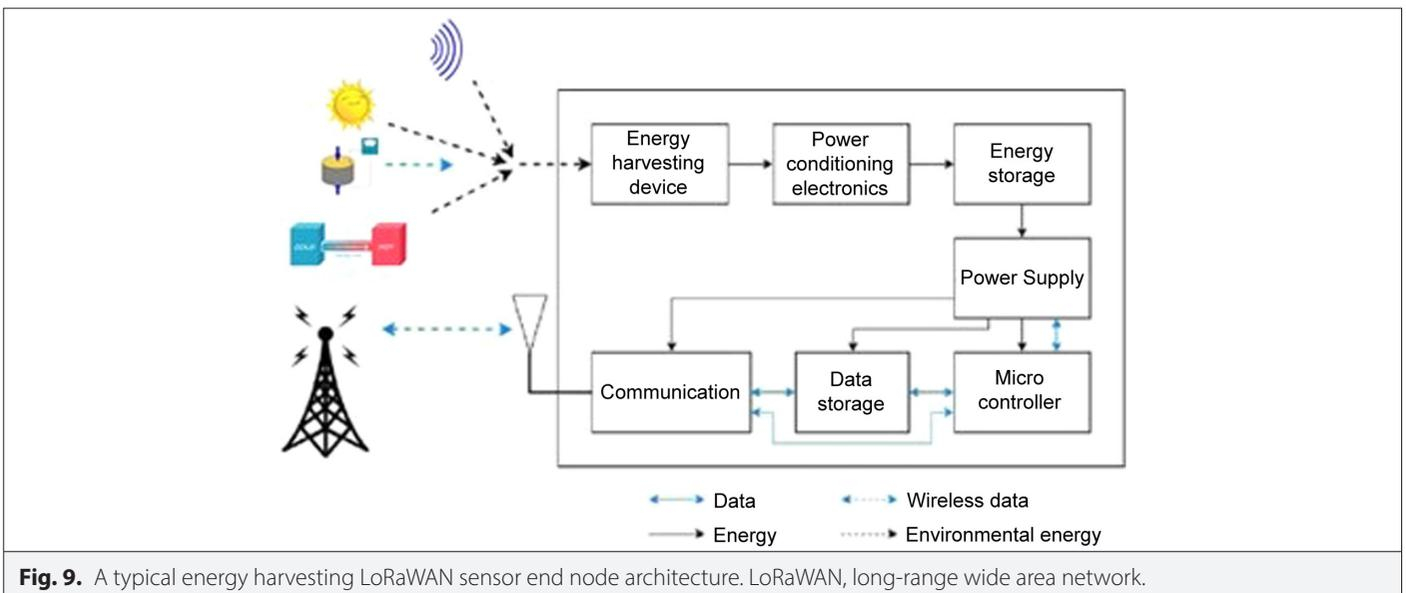
**Fig. 9.** A typical energy harvesting LoRaWAN sensor end node architecture. LoRaWAN, long-range wide area network.
