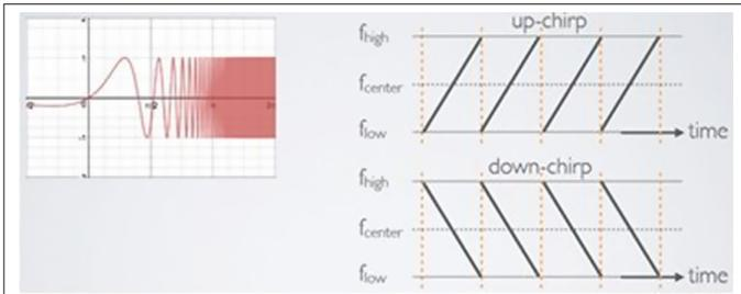
Fig. 1. Chirp-spread-spectrum (CSS) modulation.
