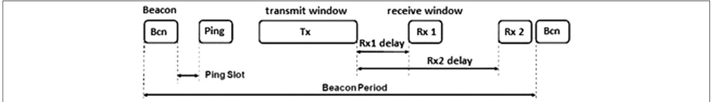
Fig. 6. Transmit and receive windows for class B device.
