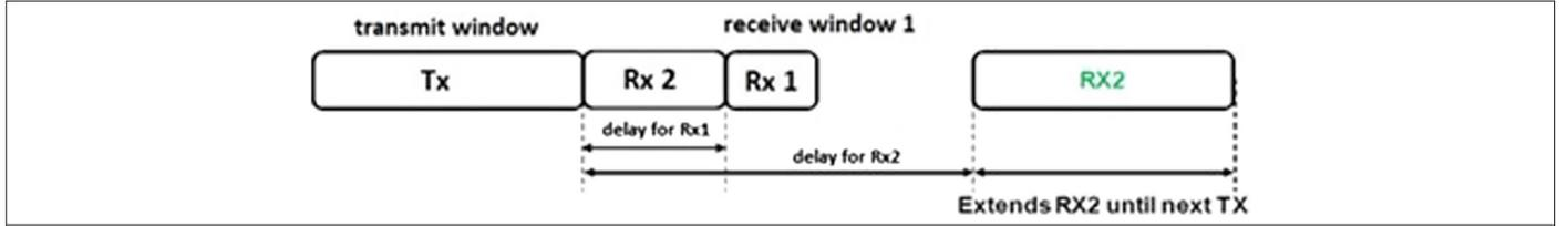
Fig. 7. Transmit and receive windows for class C device.
