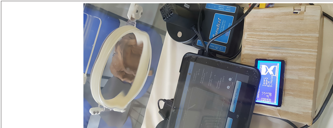
Fig. 7. Testing our device in a Drager Isolette Infant Incubator with a Datrend IncuTest incubator Tester.
