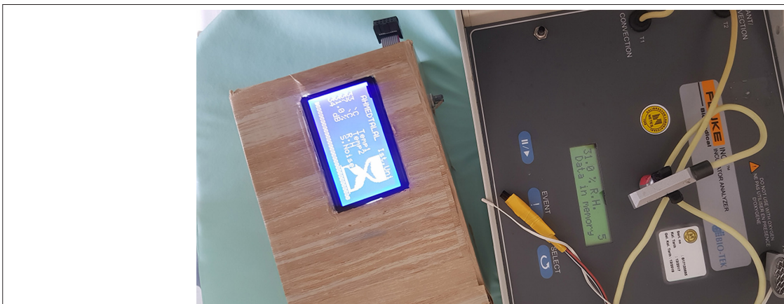
Fig. 8. Testing our device in Girffe OmniBed Infant Incubator with an INCU Fluke incubator analyzer.
