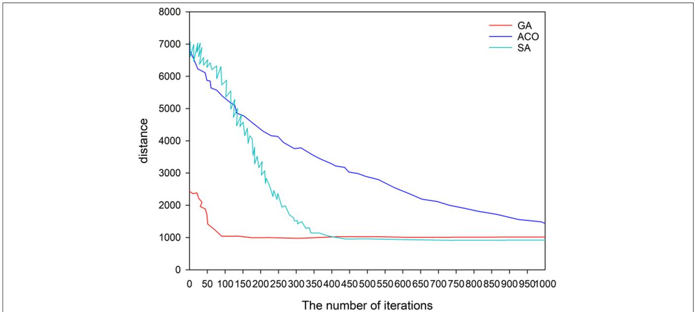
Fig. 1. Convergence of the back-end algorithm of the path planning system at 277 docking points.
