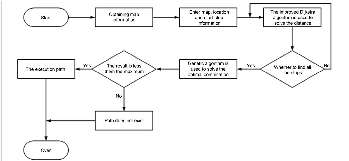
**Fig. 2.** Workflow of the path planning system.
