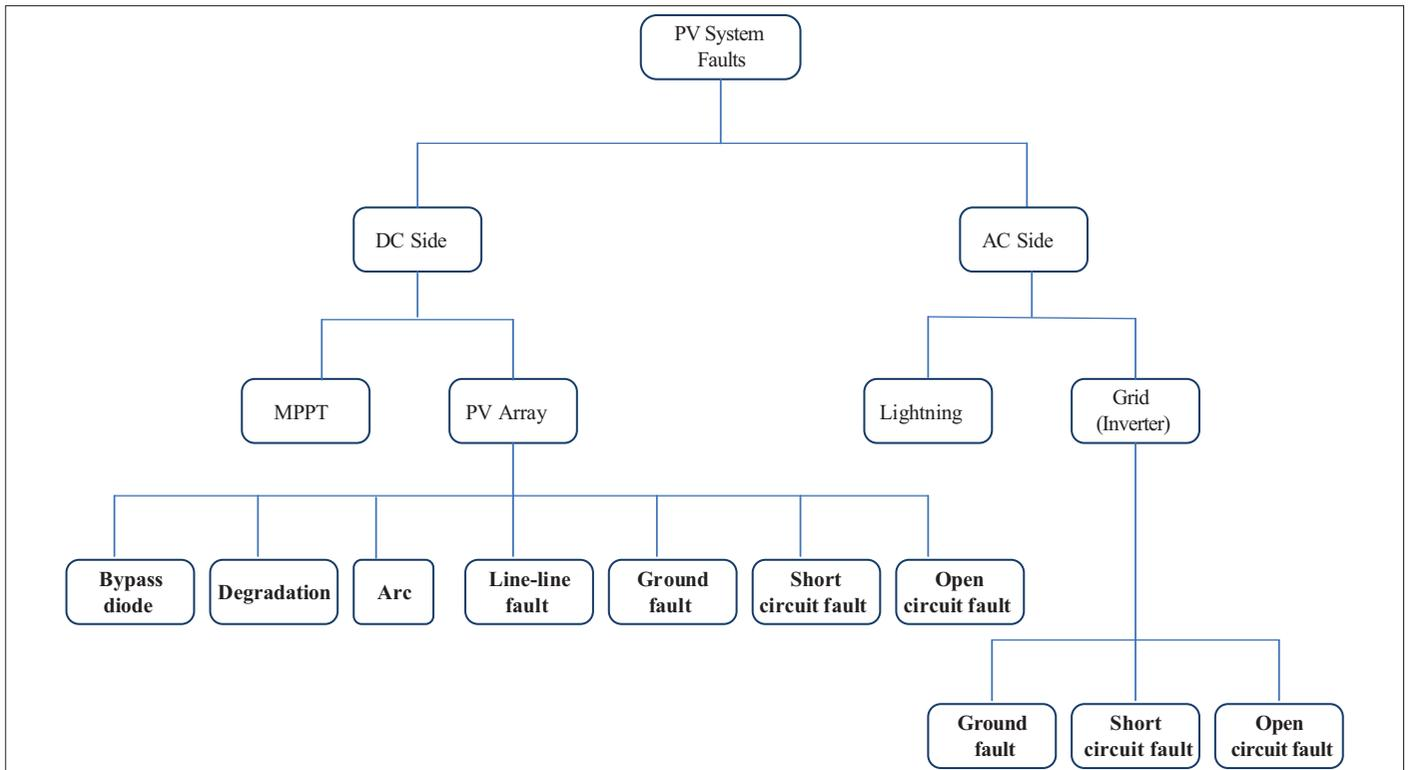
Fig. 1. Common faults on the DC and AC sides of the PV system.
