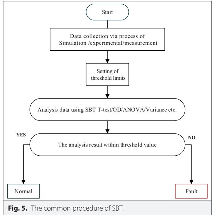
**Fig. 5.** The common procedure of SBT.
