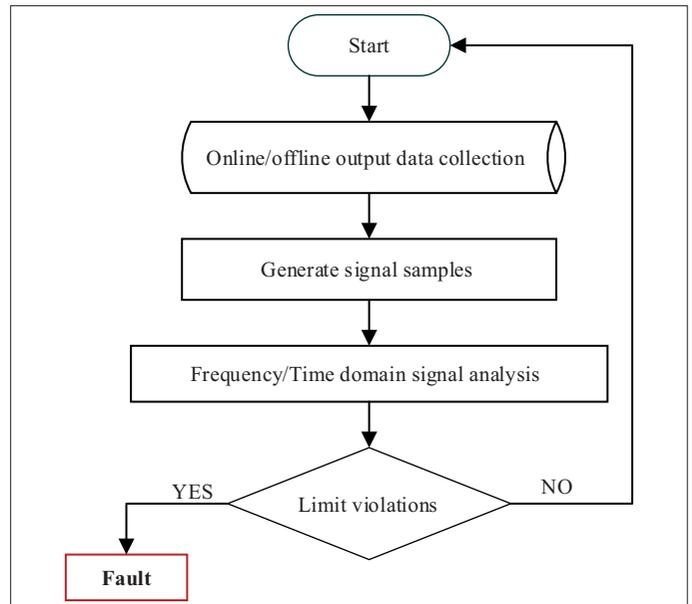
**Fig. 6.** The common procedure of OST.
