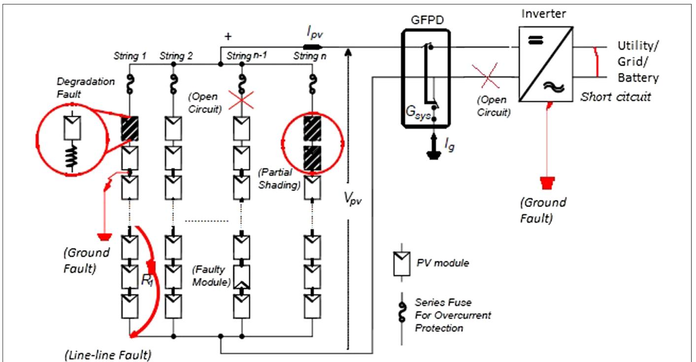
Fig. 2. Brief description of common faults on DC and AC sides of the PV system.
