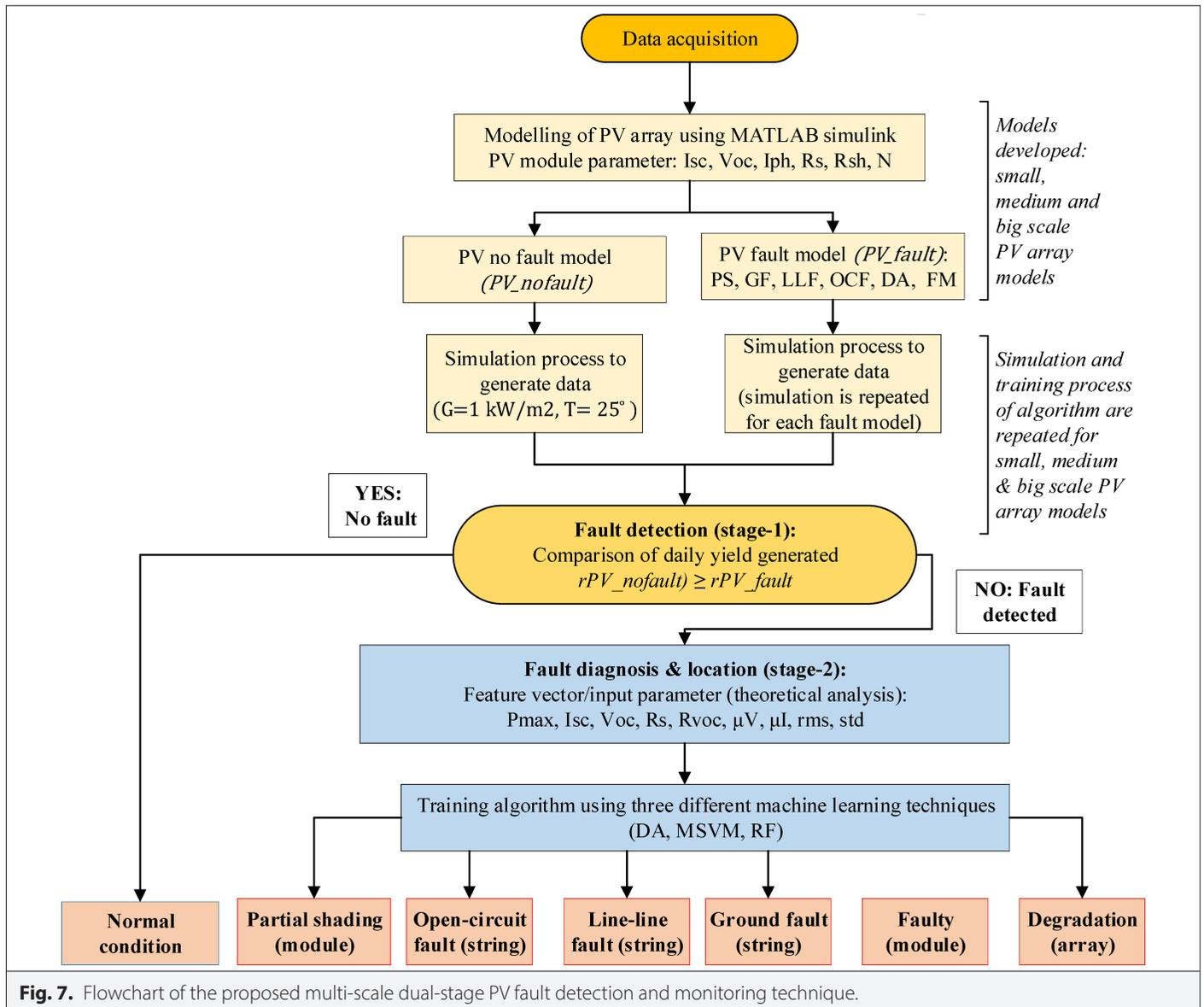
**Fig. 7.** Flowchart of the proposed multi-scale dual-stage PV fault detection and monitoring technique.
