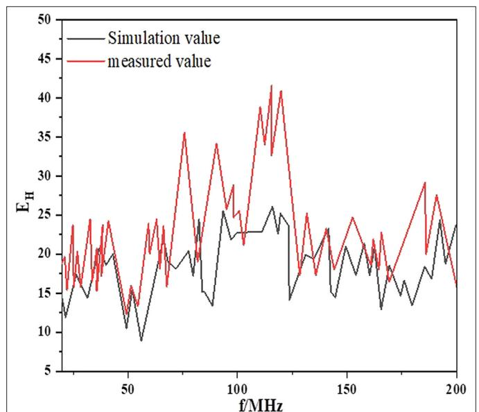
**Fig. 6.** Test results and simulation results of the vertical component of electric field intensity.
