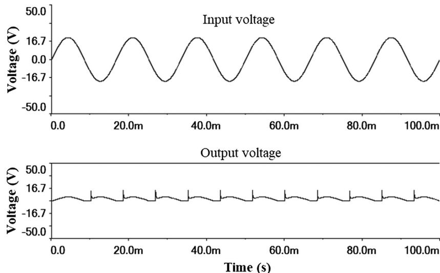
Fig. 8. Outcomes of the proposed model without electromagnetic interference filter topology.
