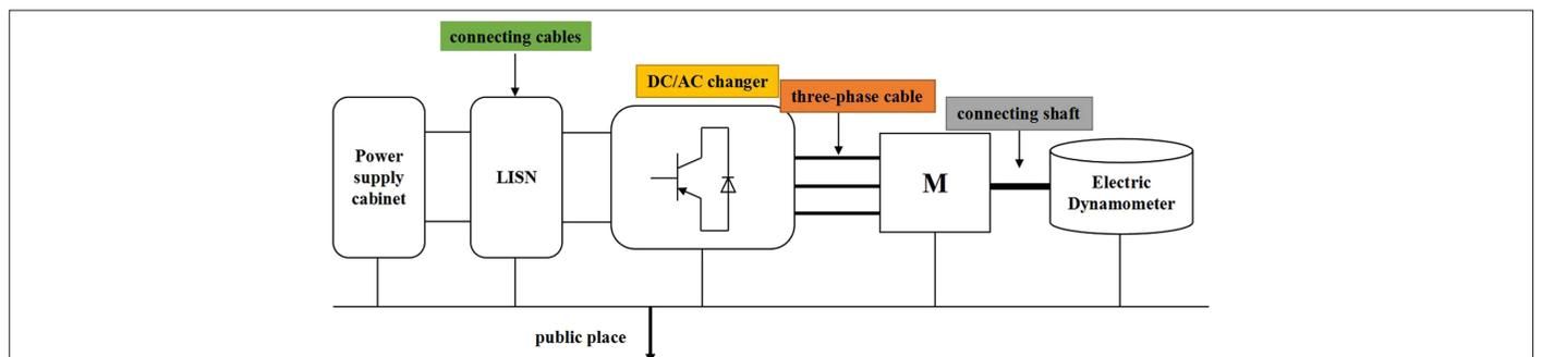
Fig. 2. Schematic diagram of a motor drive system.
