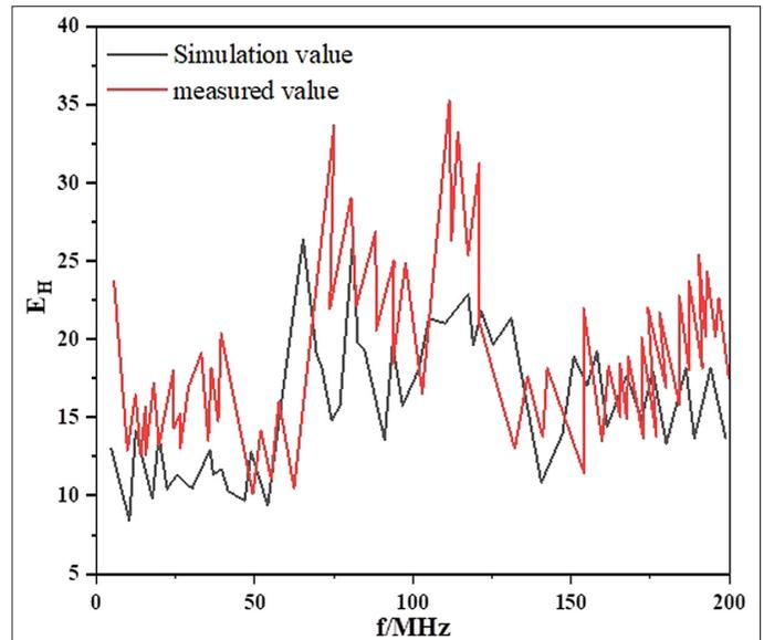
**Fig. 5.** Test results and simulation results of the horizontal component of electric field intensity.
