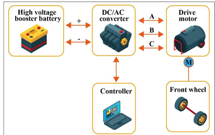
Fig. 1. Structure diagram of a motor drive system.
