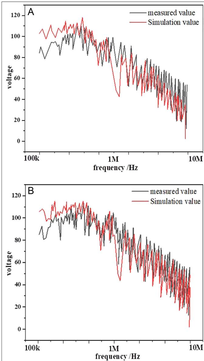
**Fig. 4.** Comparison between LISN common mode voltage simulation and measurement.
