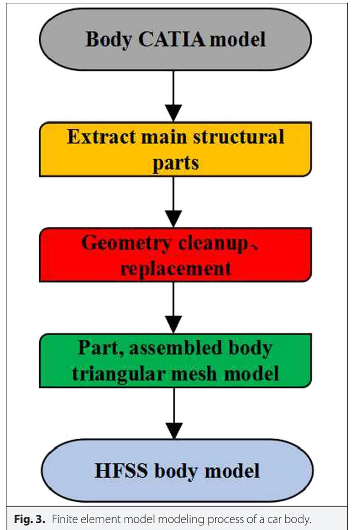
Fig. 3. Finite element model modeling process of a car body.
