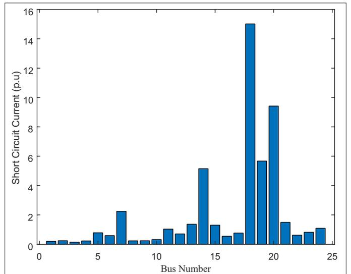
Fig. 5. Three-phase short-circuit current level in the presence of FCLs.
