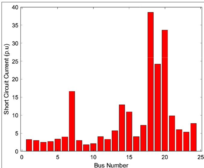
Fig. 4. Three-phase short-circuit current level without FCLs.
