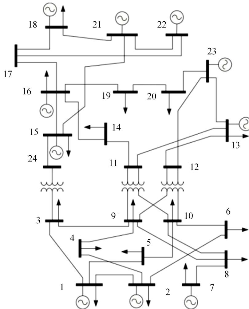
Fig. 1. Single line diagram of IEEE RTS 24-Bus system.
