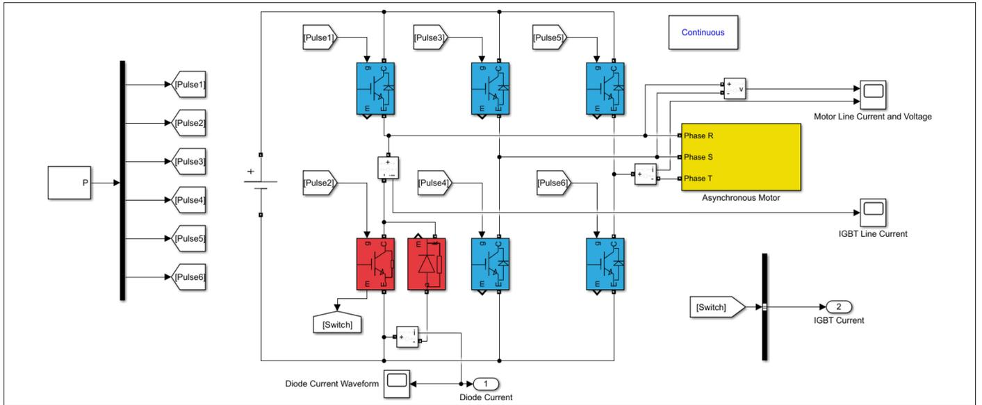
Fig. 1. MATLAB/Simulink model for an industrial motor driver.
