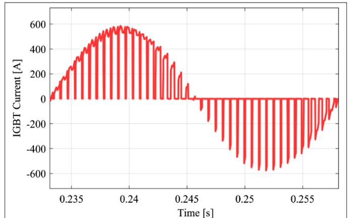
Fig. 3. Waveform of a current flowing through the insulated-gate bipolar transistor (IGBT).
