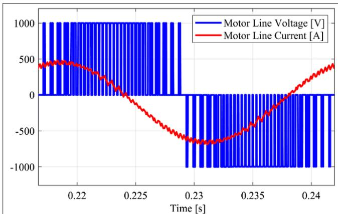
Fig. 2. Waveform of motor line voltage and current.
