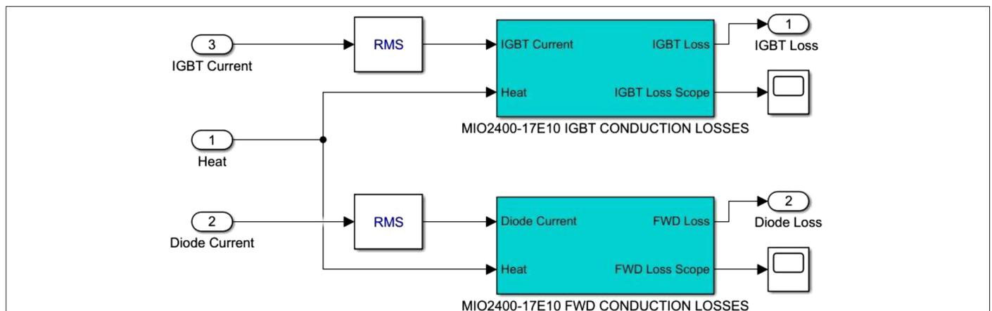
Fig. 6. Subsystem of total insulated-gate bipolar transistor (IGBT) and diode conduction loss calculation.
