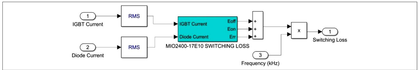
Fig. 5. Subsystem of total switching loss calculation. IGBT, insulated-gate bipolar transistor.
