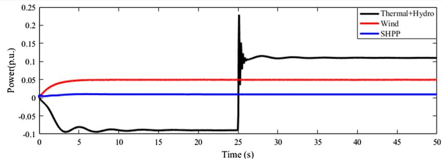
**Fig. 13.** Dynamic response of power RES in isolated mode.
