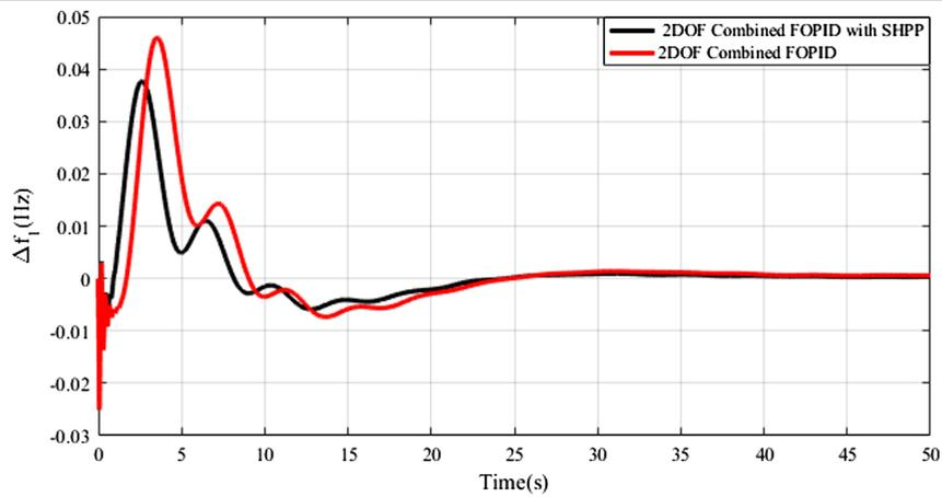
Fig. 10. Frequency deviation in area-2 with wind and SHPP (Hz).
