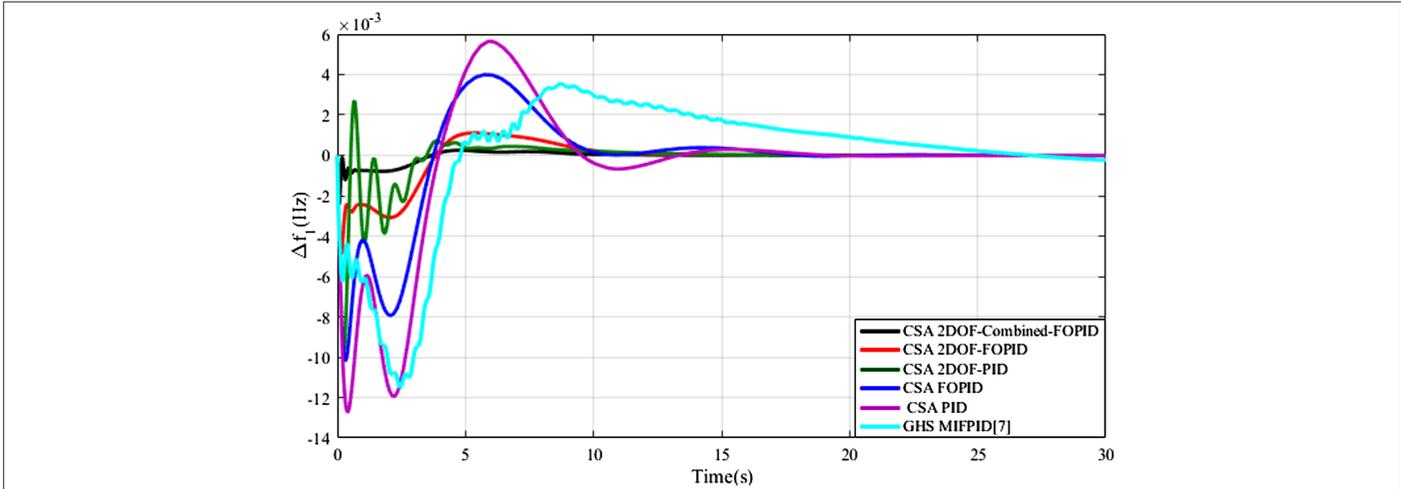
Fig. 3. Frequency deviation in area-1 (Hz).
