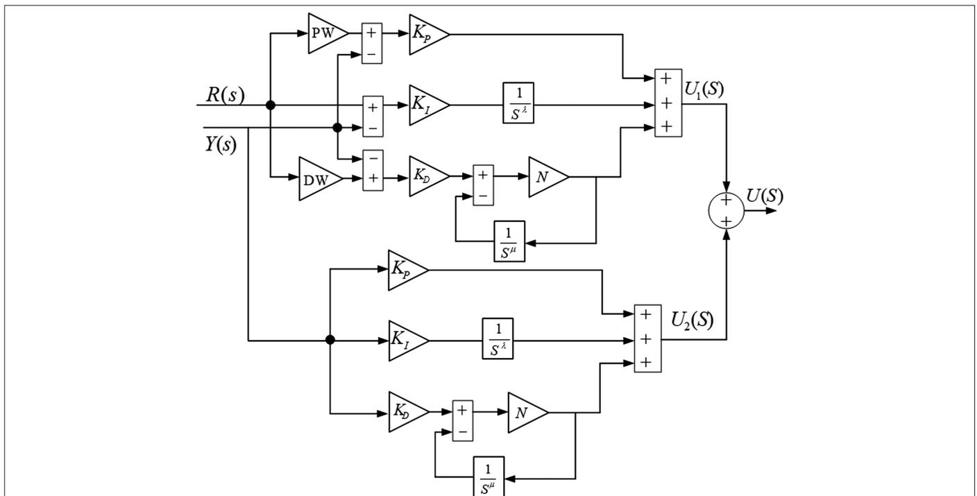
Fig. 2. 2DOF-combined FOPID controller structure. DOF, degree-of-freedom; FOPID, fractional order PID.
