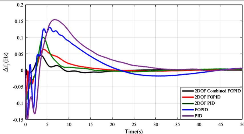
**Fig. 6.** Frequency deviation in area-1 with wind penetration (Hz).
