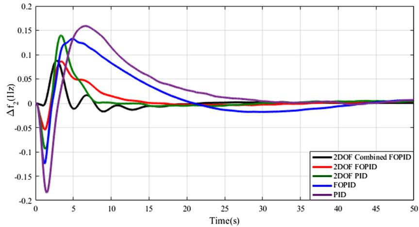
**Fig. 7.** Frequency deviation in area-2 with wind penetration (Hz).
