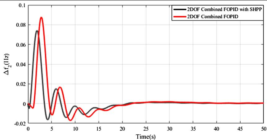
Fig. 11. Tie-line power deviation with wind and SHPP (p.u.). SHPP, small hydropower plant.
