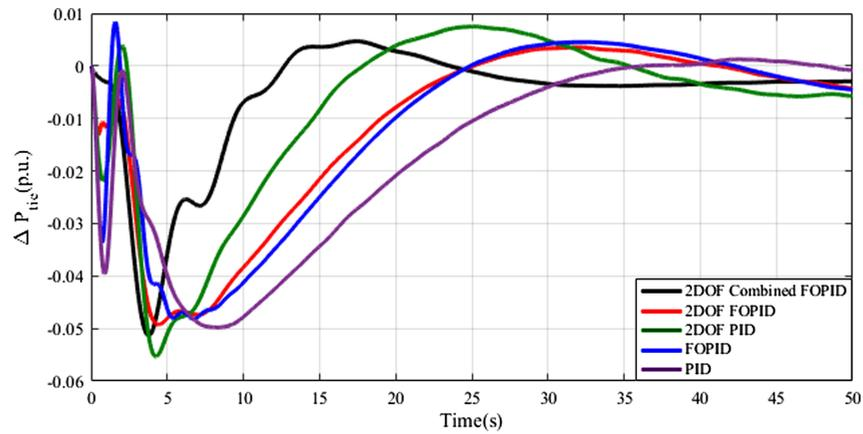
**Fig. 8.** Tie-line power deviation with wind penetration (p.u.).
