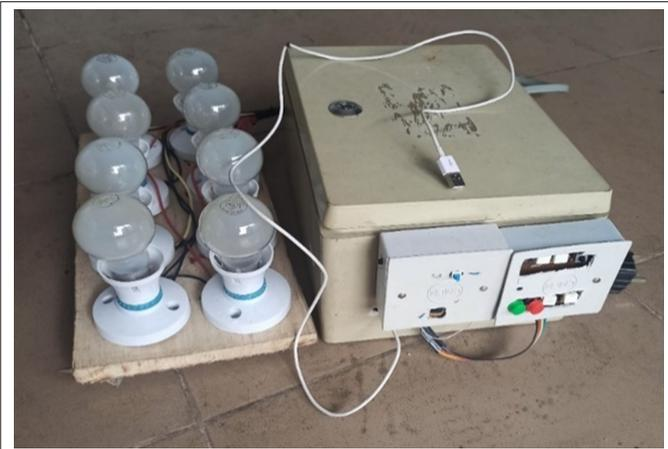
**Fig. 6.** The prototype of the smart distribution board with visitor check.
