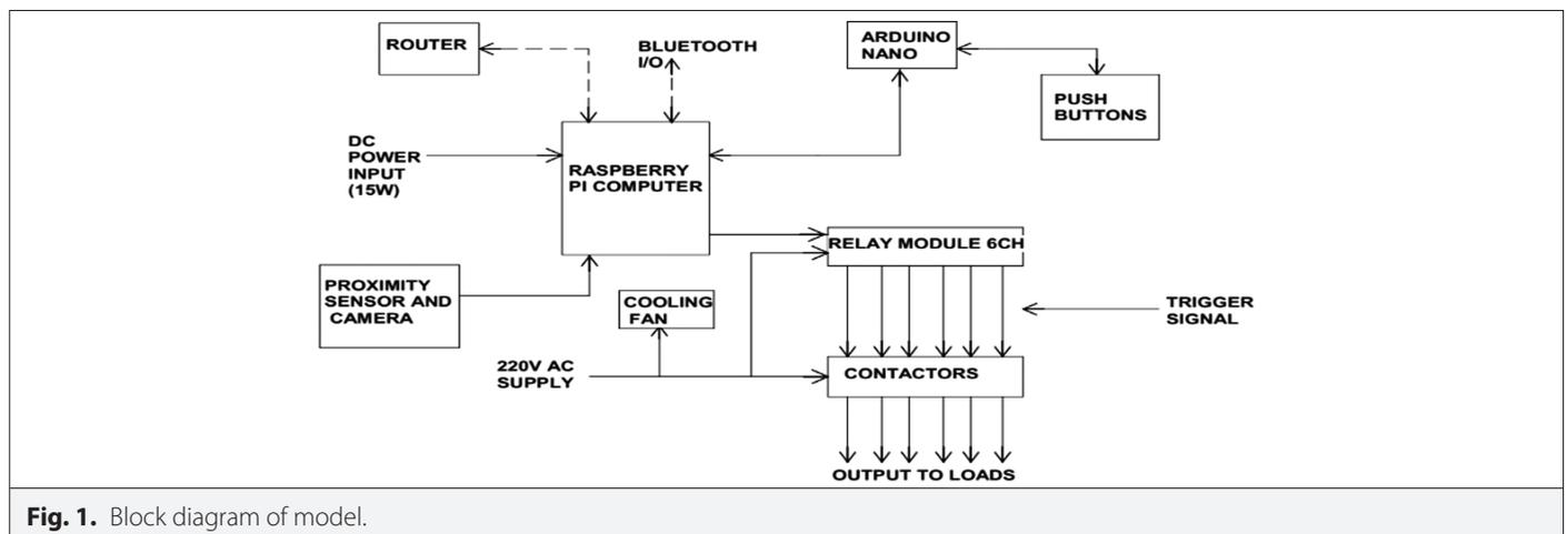
Fig. 1. Block diagram of model.
