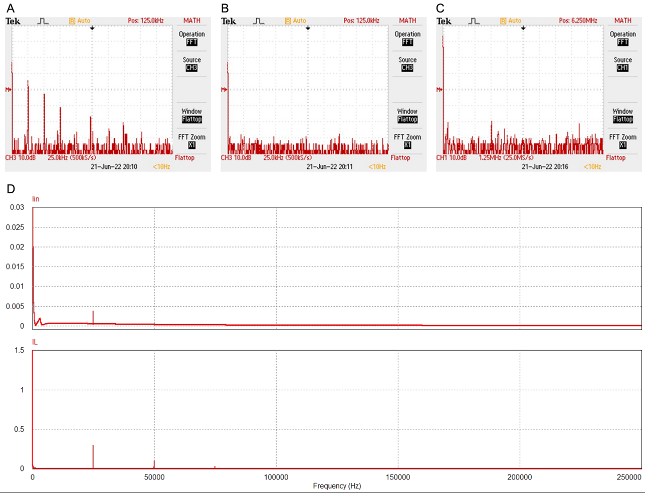
Fig. 12. (A) i_{L1} at 25 kHz, (B) i_{in} at 25 kHz, (C) DM at 1.25 MHz, and (D) FFT simulation results with a pi filter.
