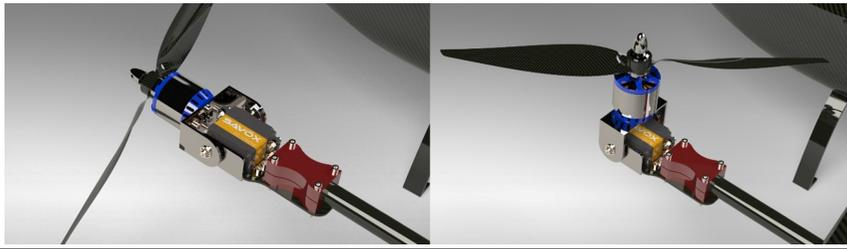
**Fig. 8.** Tilt mechanism.
