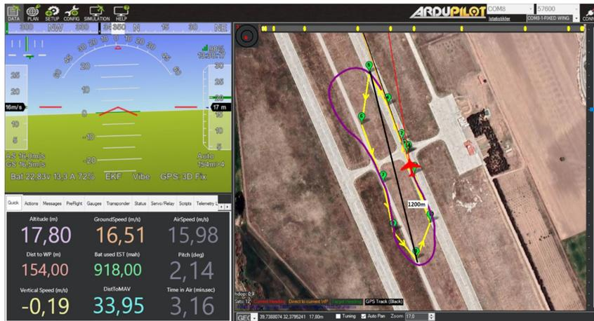
**Fig. 16.** Mission assignment and route analysis of the developed VTOL-UAV.
