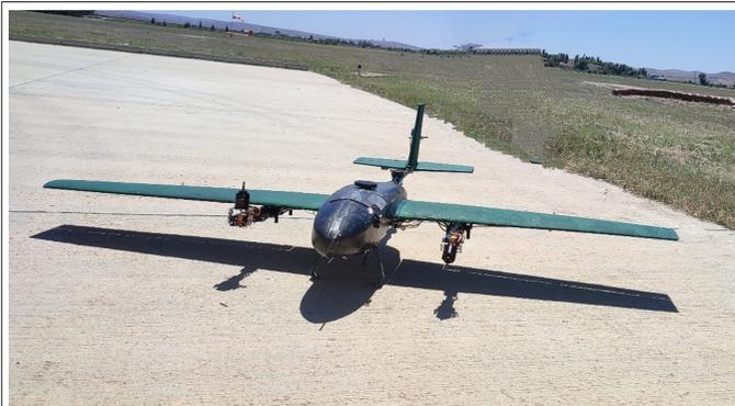
**Fig. 17.** The prototyped VTOL-UAV.
