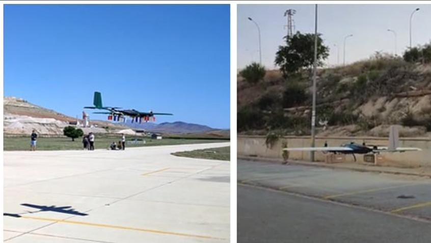
**Fig. 18.** Medical payload boxes carried on the wings of the developed UAV.
