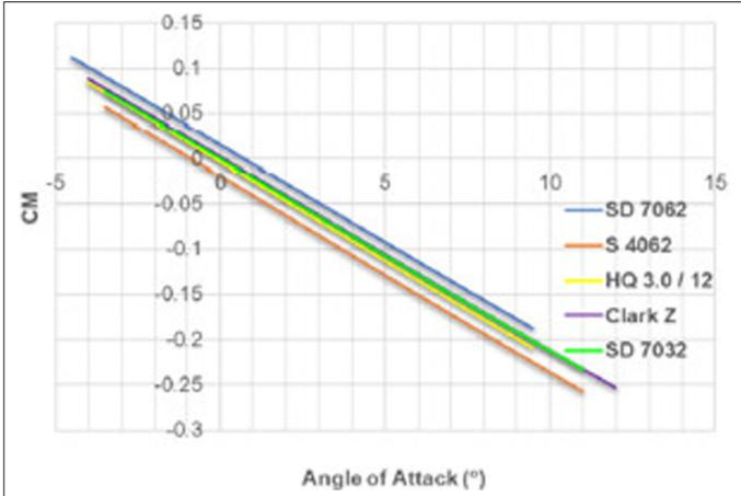
**Fig. 3.** Static stability analysis. CM, pitching moment coefficient.
