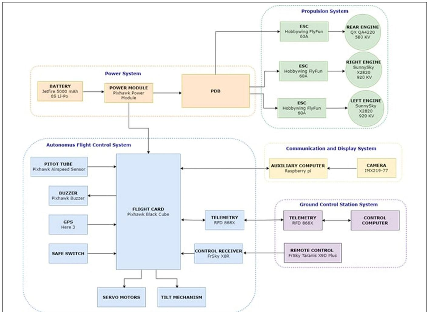
**Fig. 9.** The system architecture of the developed VTOL-UAV. ESC, electronic speed controllers; GPS, Global Positioning System; PDB, power distribution board.
