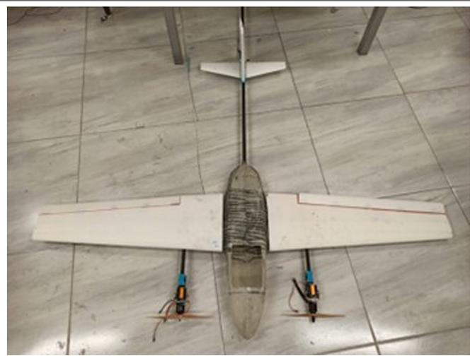
**Fig. 12.** Tilt mechanisms mounted on the VTOL-UAV fuselage.
