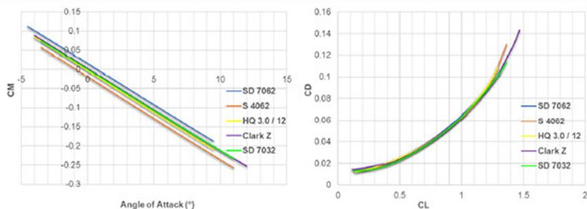
**Fig. 2.** CM vs. angle of attack and CD vs. CL charts. CD, drag coefficient; CL, lift coefficient; CM, pitching moment coefficient.
