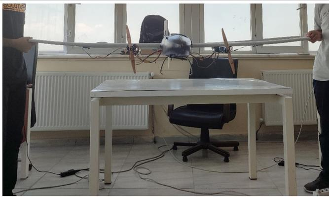
Fig. 13. Wing structural test.
