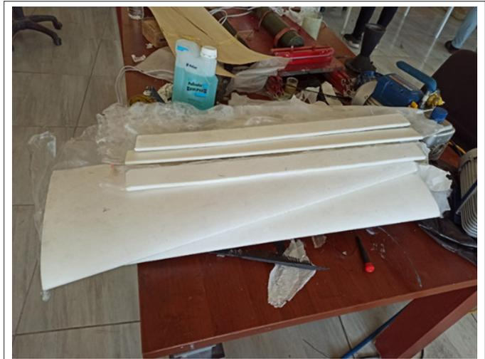
Fig. 10. Covering the wings with fiberglass.
