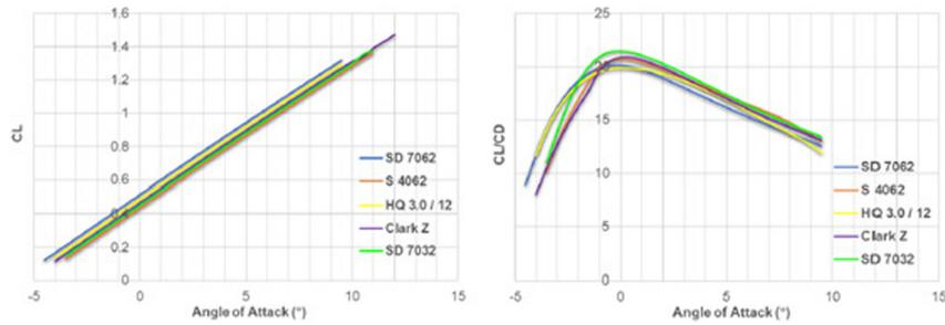
**Fig. 1.** CL vs. angle of attack and CL/CD vs. angle of attack charts. CD, drag coefficient; CL, lift coefficient.
