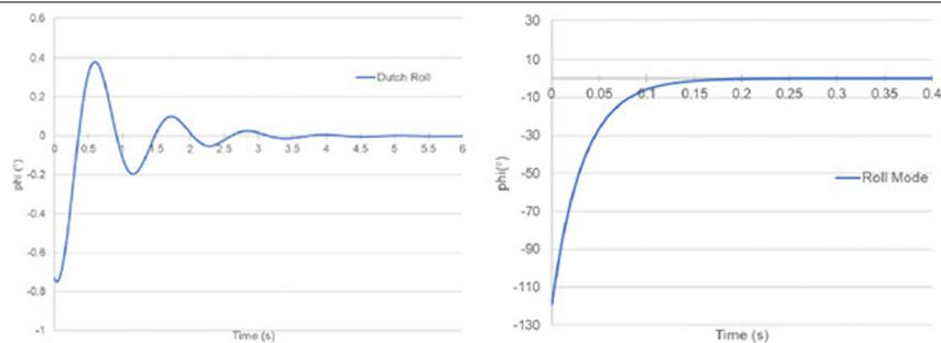
**Fig. 5.** The variations of the Dutch roll and the roll modes in time.
