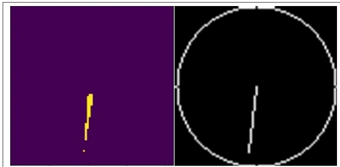
Fig. 8. Input (left) and calculated output (right) for the needle mask task, which was -96.70^\circ .
