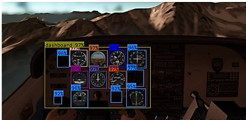
Fig. 5. YOLOv8 prediction on a sample. All dials were correctly classified with the annotated confidence scores.
