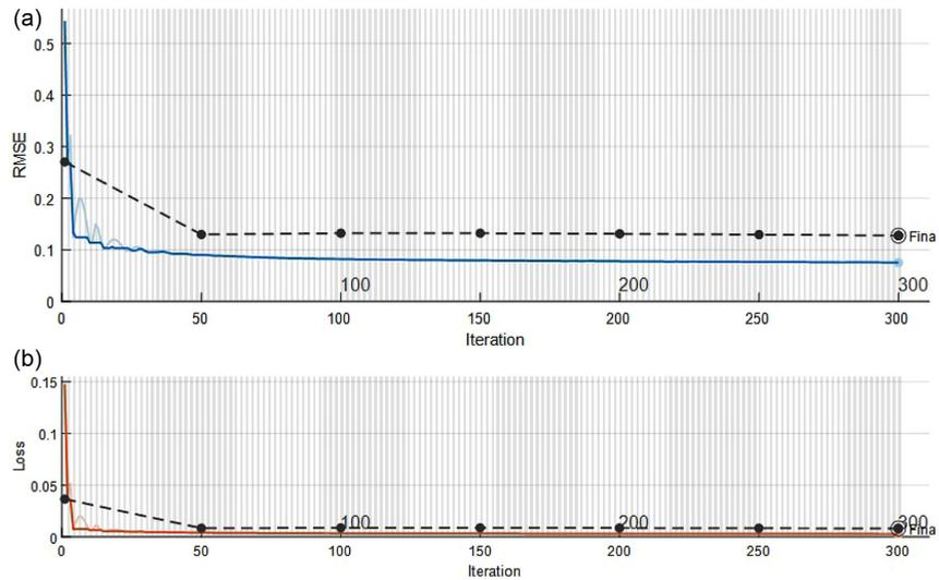
**Fig. 12.** (a) RMSE value curve of LSTM model during training and (b) loss function curve of LSTM model during training (dotted line = validation, smooth line = train).
