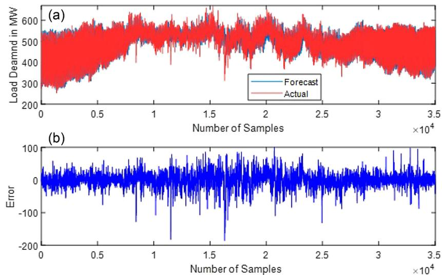
**Fig. 13.** During training of LSTM for the 2022 year dataset. (a) Actual and predicted load. (b) Error.
