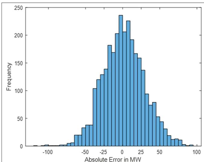
**Fig. 6.** Error histogram of load prediction during testing of GPR with January 2023 dataset.
