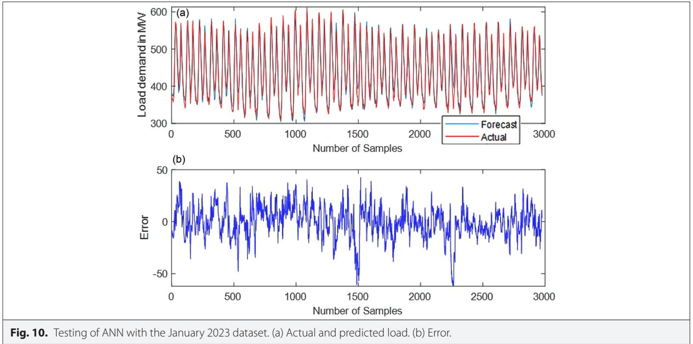
**Fig. 10.** Testing of ANN with the January 2023 dataset. (a) Actual and predicted load. (b) Error.
