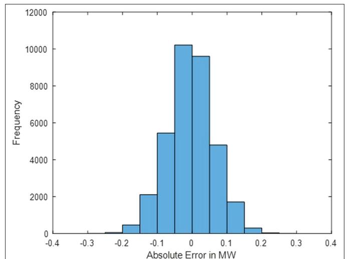
**Fig. 4.** Error histogram of load prediction during training of GPR-based LF model for the year 2022 dataset.
