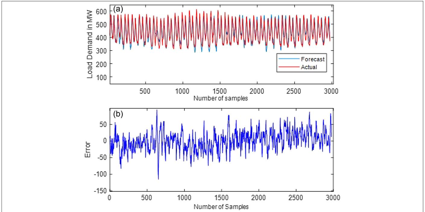
**Fig. 5.** Testing of GPR-based LF model with January 2023 dataset. (a) Actual and predicted load. (b) Error.
