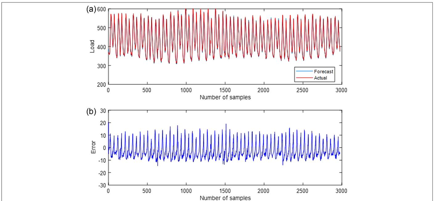
**Fig. 15.** During testing of LSTM with January 2023 dataset. (a) Actual and predicted load. (b) Error.
