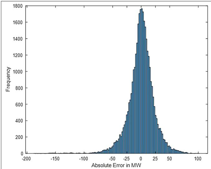
**Fig. 14.** Absolute error histogram of load prediction during training of LSTM for the year 2022 dataset.
