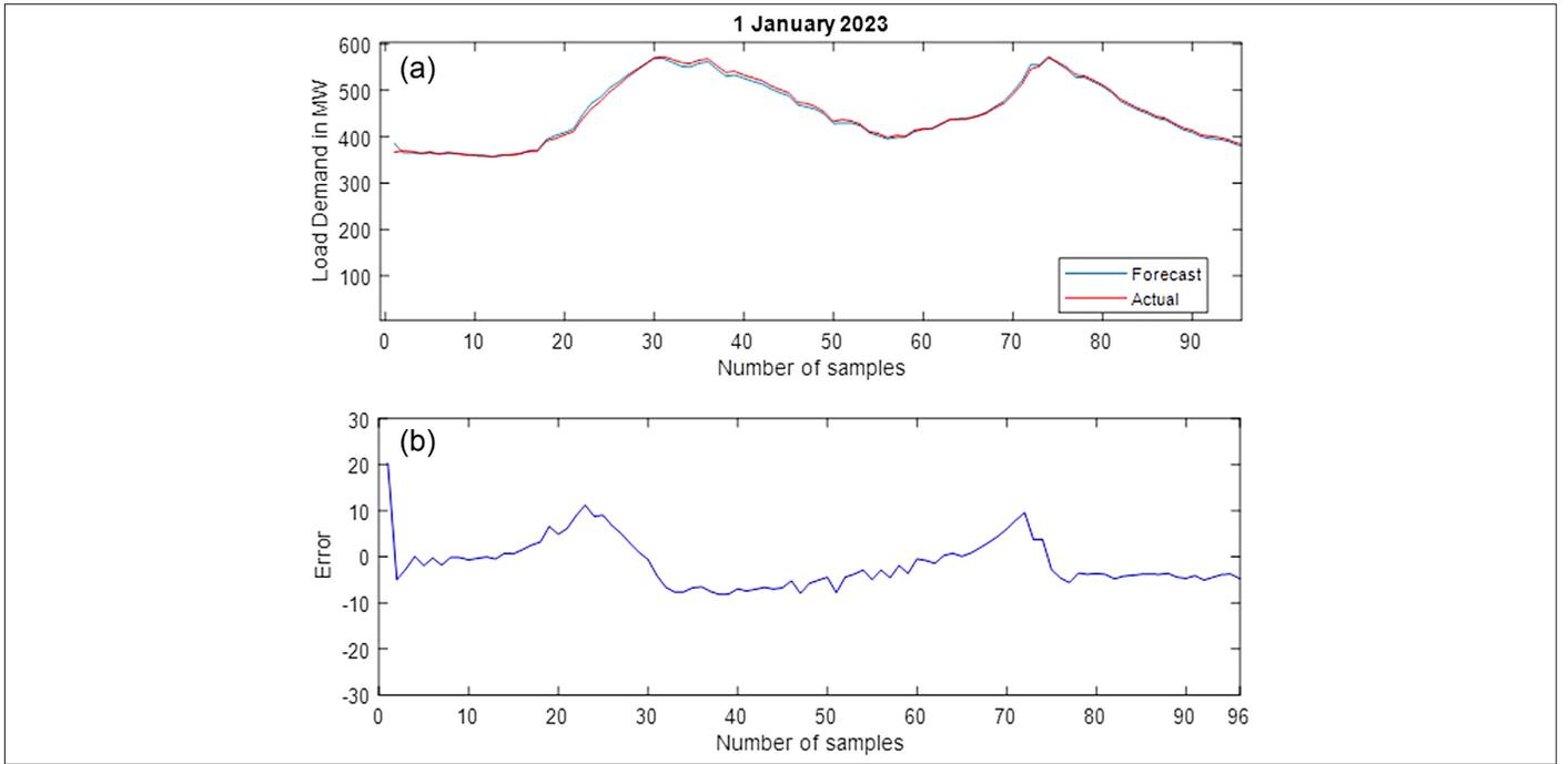
**Fig. 17.** On 1st January 2023. (a) Actual and predicted load plot and (b) error.
