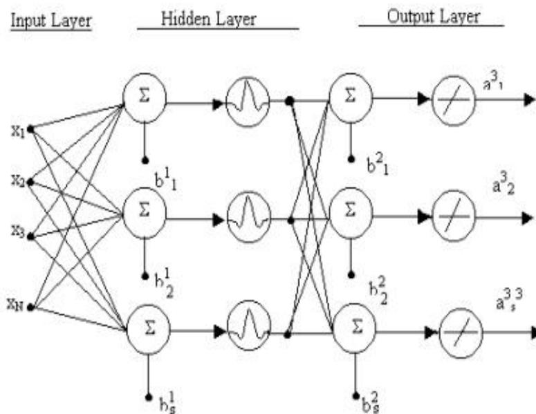
Fig. 1. Wavelet Neural Network architecture
