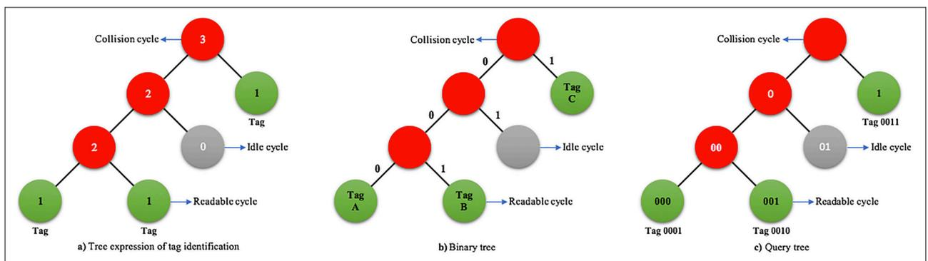
Figure 6. Tag identification in tree-based protocols
