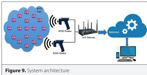
Figure 9. System architecture
