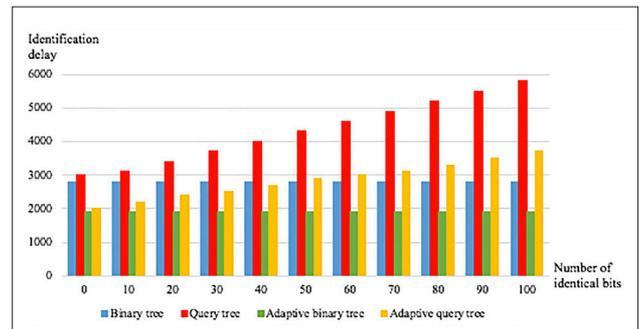
Figure 15. Identification delay by tag ID similarity
