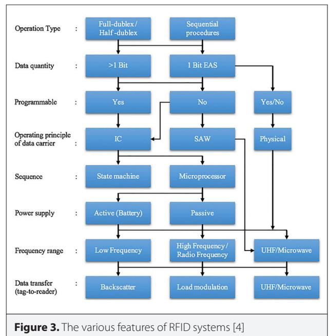
Figure 3. The various features of RFID systems [4]
