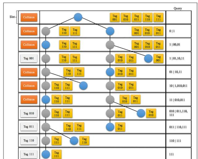
Figure 8. Tag identification using the query tree protocol
