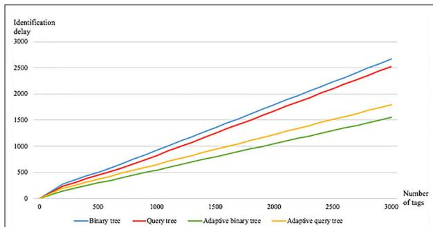
Figure 12. Identification delay by the number of tags
