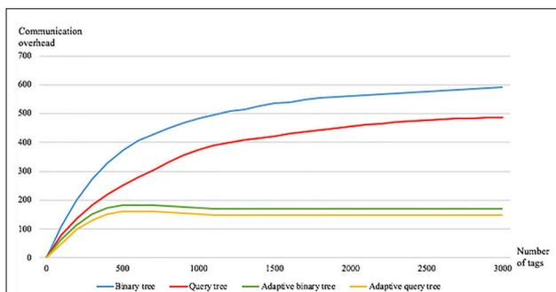
Figure 13. Communication overhead by the number of tags
