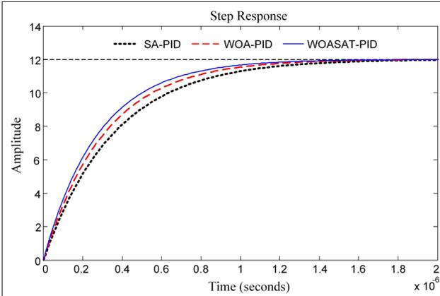
**Figure 9.** Step response comparisons of the buck converter system
