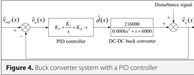
Figure 4. Buck converter system with a PID controller
