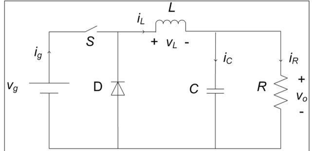
Figure 1. Buck converter system without of any controller
