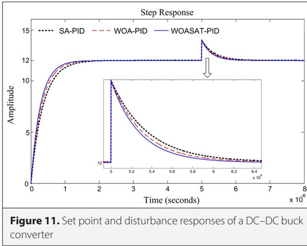
**Figure 11.** Set point and disturbance responses of a DC-DC buck converter
