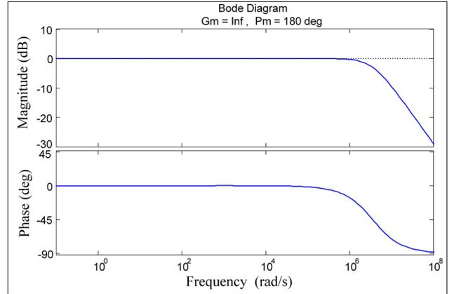
**Figure 10.** Bode plot of the buck converter system with a WOASAT-based PID controller
