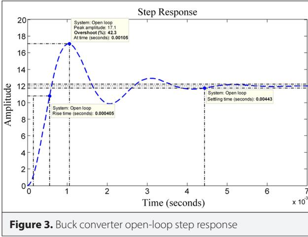
Figure 3. Buck converter open-loop step response
