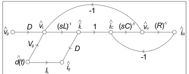
Figure 2. Buck converter small-signal (dynamic) model
