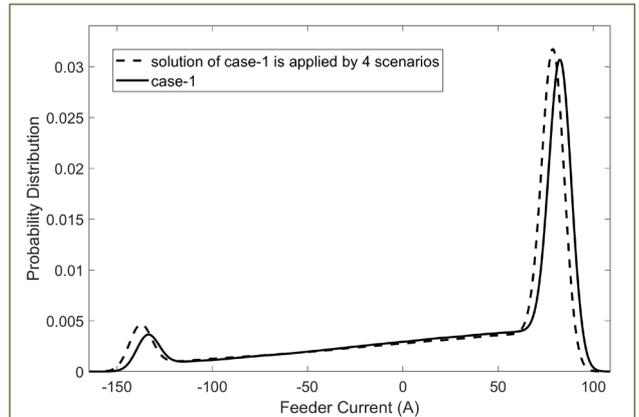
**Figure 5.** Probability distribution of feeder current between nodes 4-29 for WPP cases
