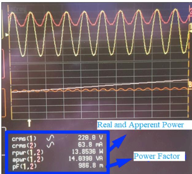
Figure 5. Input real and apparent power with PF values
