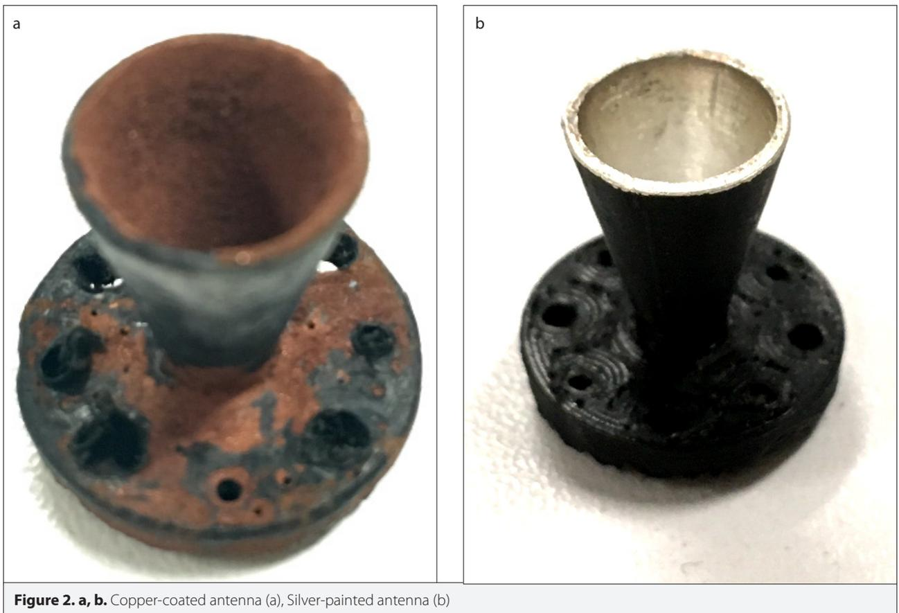
Figure 2. a, b. Copper-coated antenna (a), Silver-painted antenna (b)
