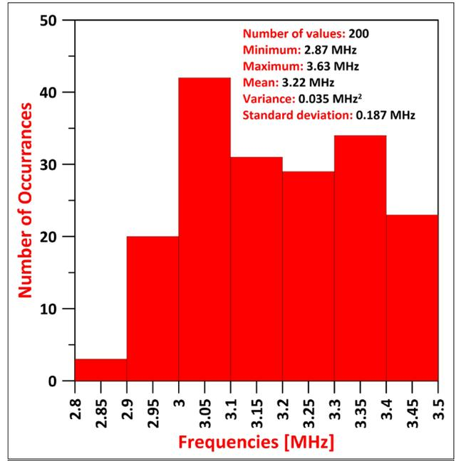
**Figure 16.** Bandwidth change obtained by changing the dimensions (W), V<sub>TH</sub> and tox parameters of MOS transistors of Monte Carlo analysis by 10%
