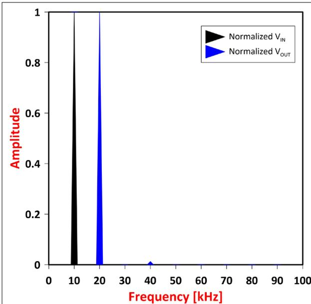
Figure 12. Frequency spectrum of the frequency doubler
