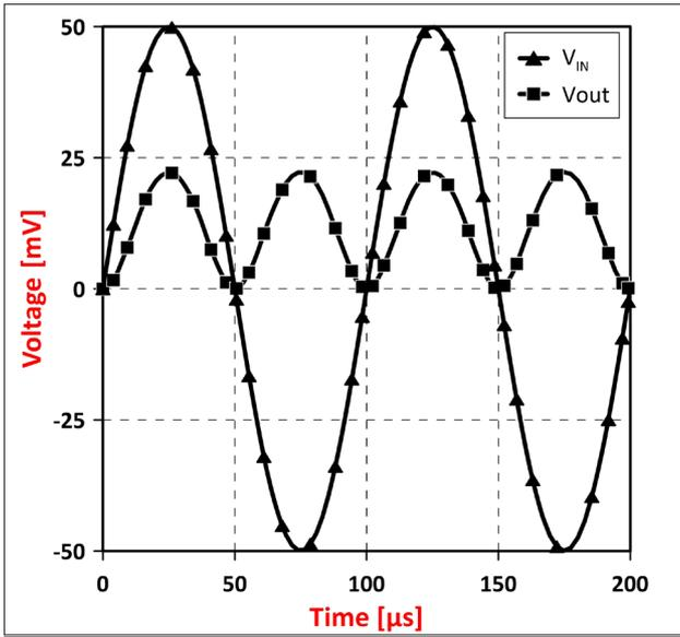
Figure 11. Input ( $V_{IN}$ ) and output ( $V_{OUT}$ ) waveforms of the frequency doubler
