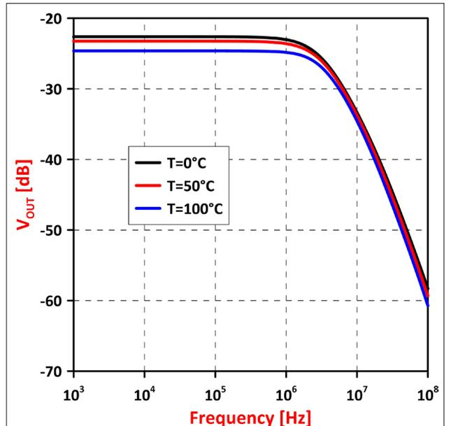
Figure 14. AC characteristics according to the temperature variation
