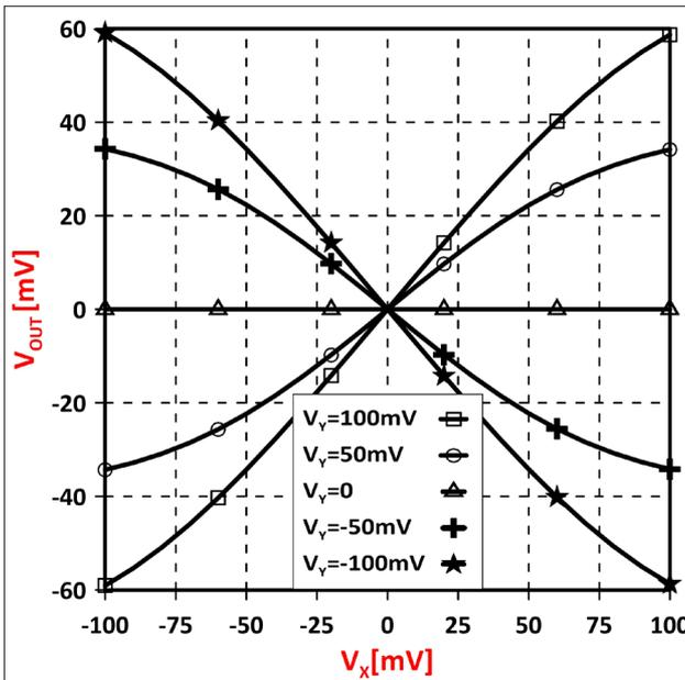
Figure 4. DC characteristic ( $V_x$  terminal).
