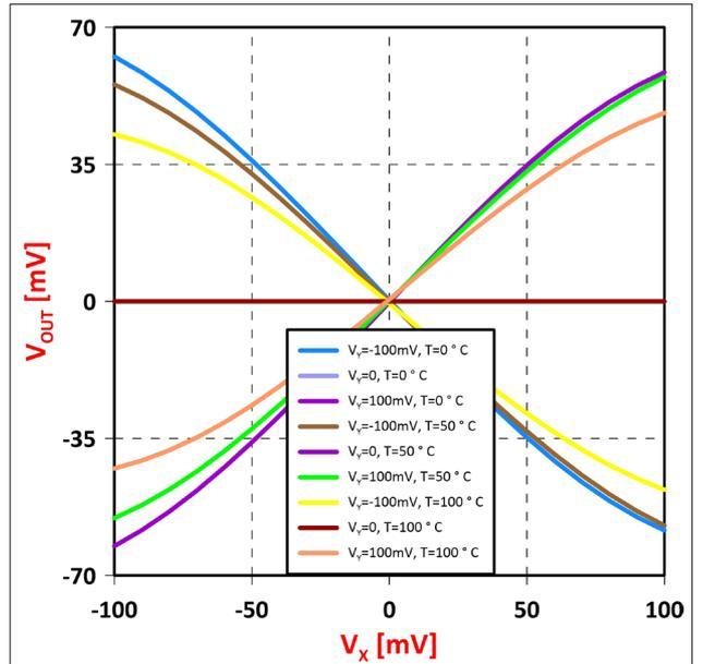
Figure 13. DC characteristics according to the temperature variation
