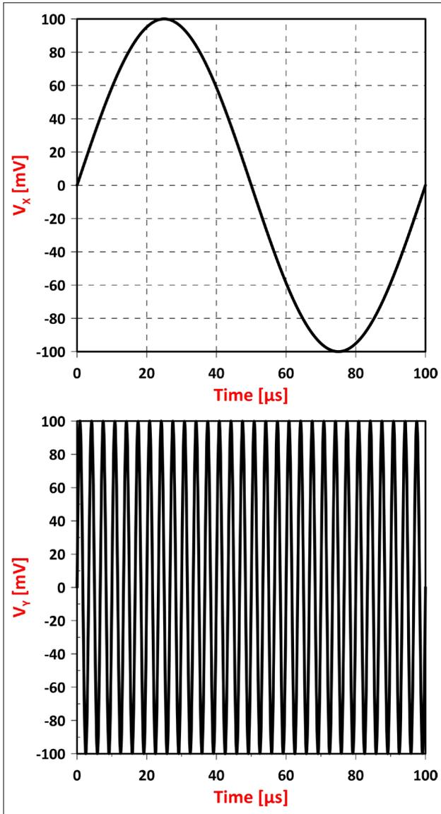
Figure 7. Input waveforms of the modulator
