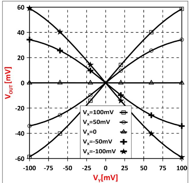
Figure 5. DC characteristic ( $V_y$  terminal)
