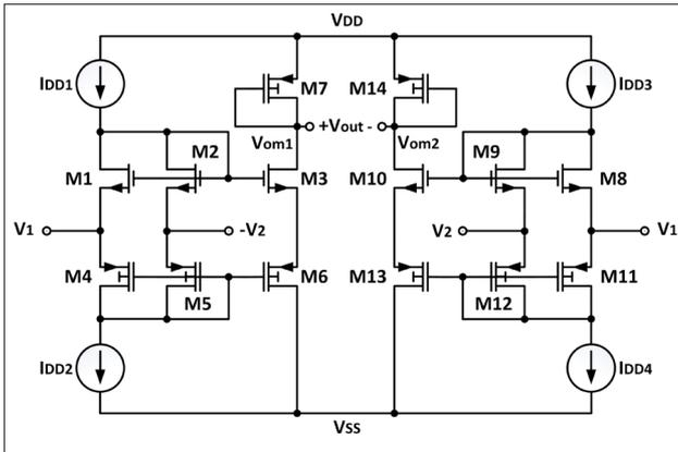
Figure 3. DTMOS based FQAM
