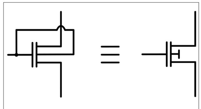
Figure 1. DTMOS circuit topology and symbol [38]
