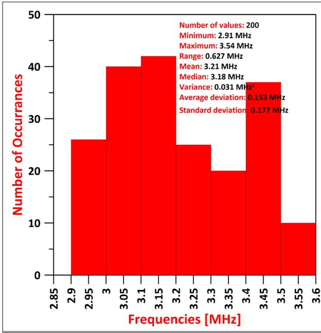
**Figure 15.** Bandwidth change obtained by changing the size (w) of MOS transistors by 10% of Monte Carlo analysis
