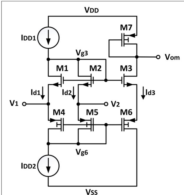
Figure 2. The basic amplifier circuit
