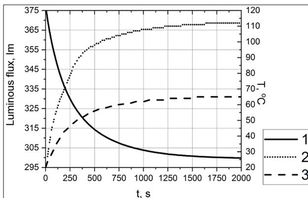
**Figure 6.** Change dynamics in the luminous flux (1), the temperature of the diode mounting board (2) and the temperature of the LED lamp casing (3) with Svetkomplekt 7W LEDs during the operation of the luminaire
