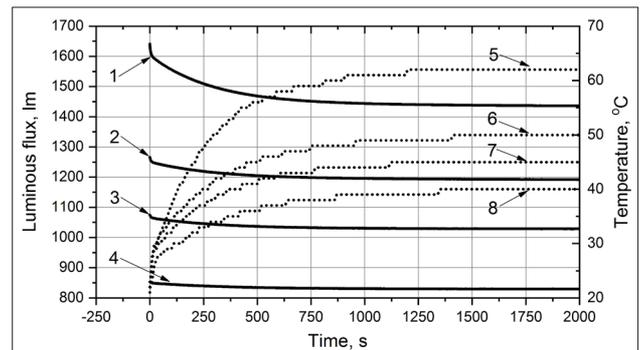
**Figure 12.** Change dynamics in luminous flux (1-4) and temperature in the zone of diode installation (5-8) in the luminaire with a cooling system based on heat pipes and a power of 32.16 W (1 and 5, respectively), 20.37W (2 and 6, respectively), 15.93W (3 and 7, respectively), 11.63W (4 and 8, respectively)
