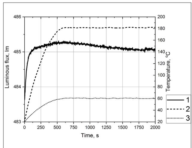
**Figure 5.** Change dynamics in the luminous flux (1), the temperature of the incandescent lamp bulb (2) and the temperature of the E14 holder(3) with 60W incandescent lamp during the operation of the luminaire
