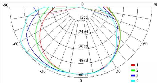
**Figure 10.** Luminous intensity indicatrices of the luminaire with installed diffusing shade for a luminaire with used three-dimensional LED module with a heat pipe for C-planes rotated to the horizon at angles: 1-0°; 2-30°; 3-60°; 4-90°
