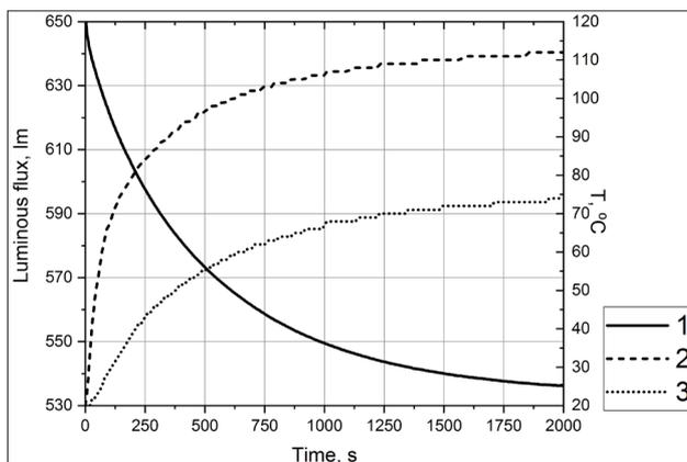
**Figure 7.** Change dynamics in the luminous flux (1), the temperature of the diode mounting board (2) and the temperature of the LED lamp casing (3) of the MAXUS 8W lamp during the operation of the luminaire
