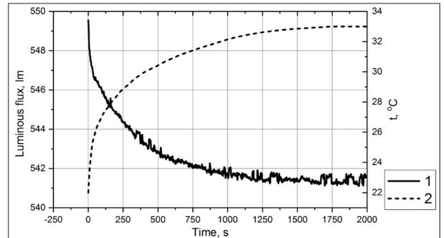
**Figure 11.** Change dynamics in luminous flux (1) and temperature in the zone of diode installation (2) in the luminaire with a cooling system based on heat pipes and a power of 6.72 W
