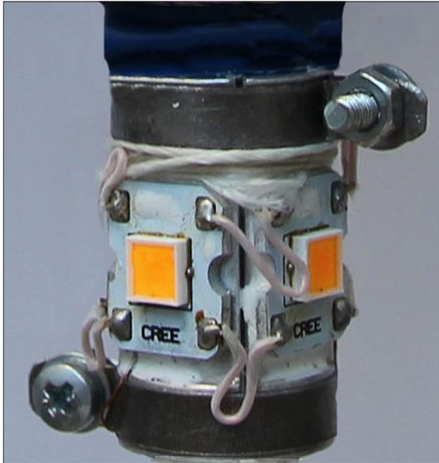
**Figure 9.** Three-dimensional LED module used in the luminaire
