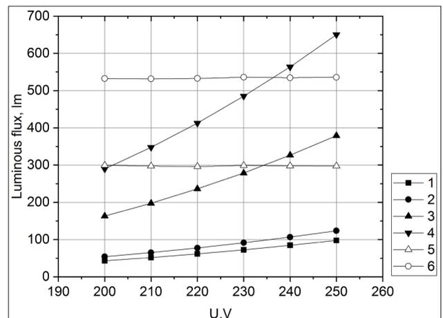
**Figure 3.** Effect of voltage change on the luminous flux of the luminaire with incandescent lamps (1 — 15 W, 2 — 25 W, 3 — 40 W, 4 — 60 W) and LED lamps (5 — Svetkomplekt 7 W, 6 — MAXUS 8W)
