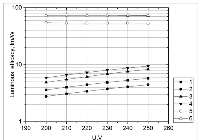
**Figure 4.** Effect of voltage change on the luminous efficacy of the lighting device with incandescent lamps (1 — 15 W, 2 — 25 W, 3 — 40 W, 4 — 60 W) and LED lamps (5 — Svetkomplekt 7 W, 6 — MAXUS 8W)
