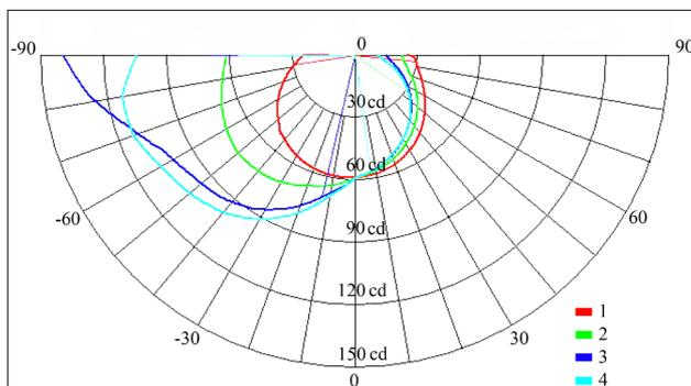
**Figure 2.** Luminous intensity indicatrices of the luminaire with installed diffusing shade for a MAXUS 8W LED lamp for C-planes rotated to the horizon at angles: 1-0°; 2-30°; 3-60°; 4-90°
