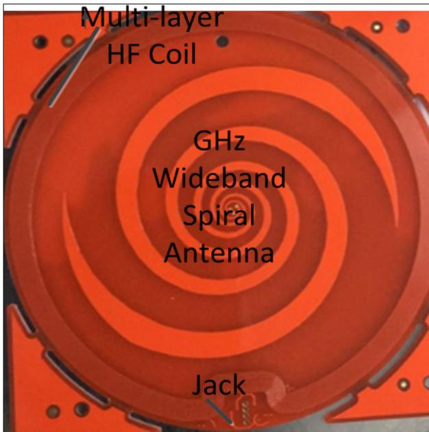
Figure 7. Top view of the electronic system PCB
