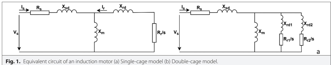
Fig. 1. Equivalent circuit of an induction motor (a) Single-cage model (b) Double-cage model.
