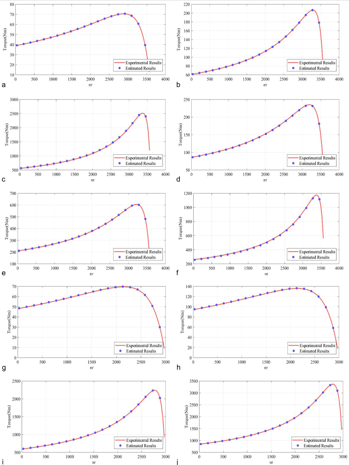
**Fig. 3.** Speed–Torque characteristics of ten different induction motors: (a) Motor 1, (b) Motor 3, (c) Motor 7, (d) Motor 10, (e) Motor 11, (f) Motor 12, (g) Motor 14, (h) Motor 15, (i) Motor 19, and (j) Motor 20.
