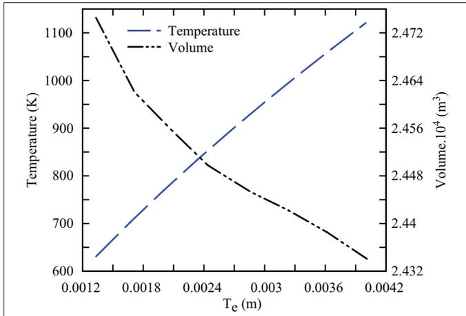
**Fig. 7.** Effect of fin's maximum thickness on the mean temperature and volume.
