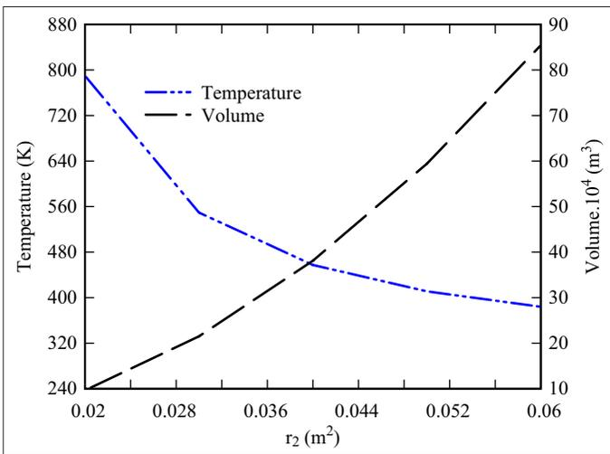
**Fig. 3.** Effect of heat sink's outer radius on the mean temperature and volume.
