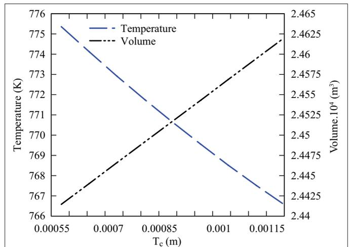
**Fig. 6.** Effect of fin's minimum thickness on the mean temperature and volume.
