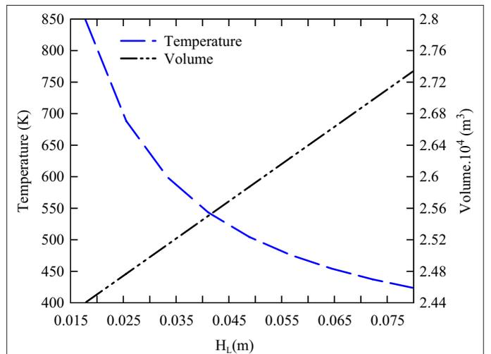
**Fig. 5.** Effect of fin's width on the mean temperature and volume.
