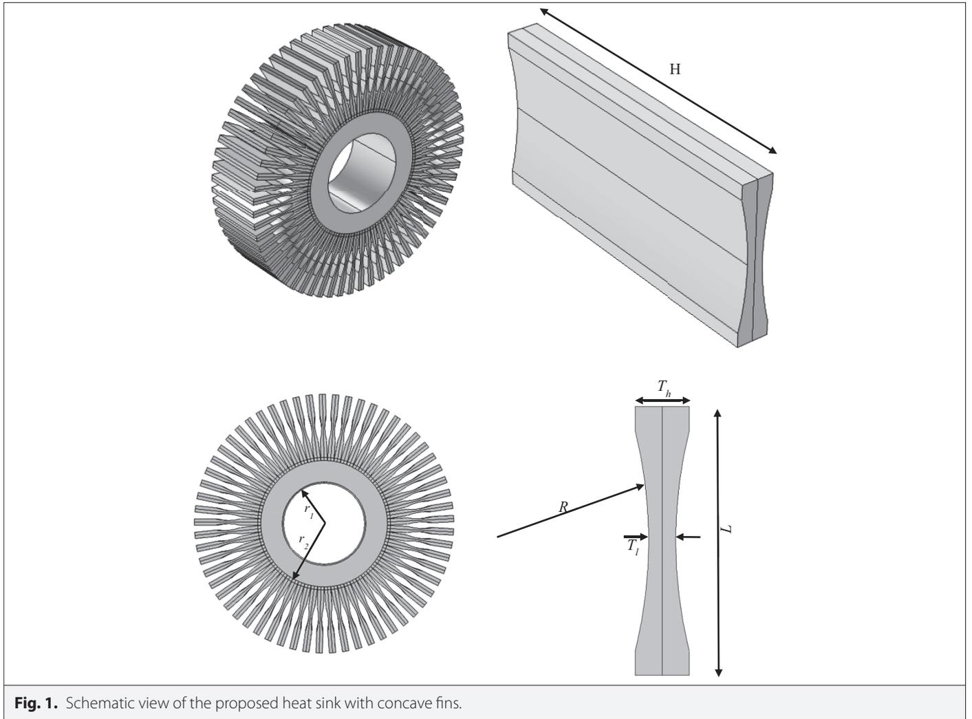
Fig. 1. Schematic view of the proposed heat sink with concave fins.
