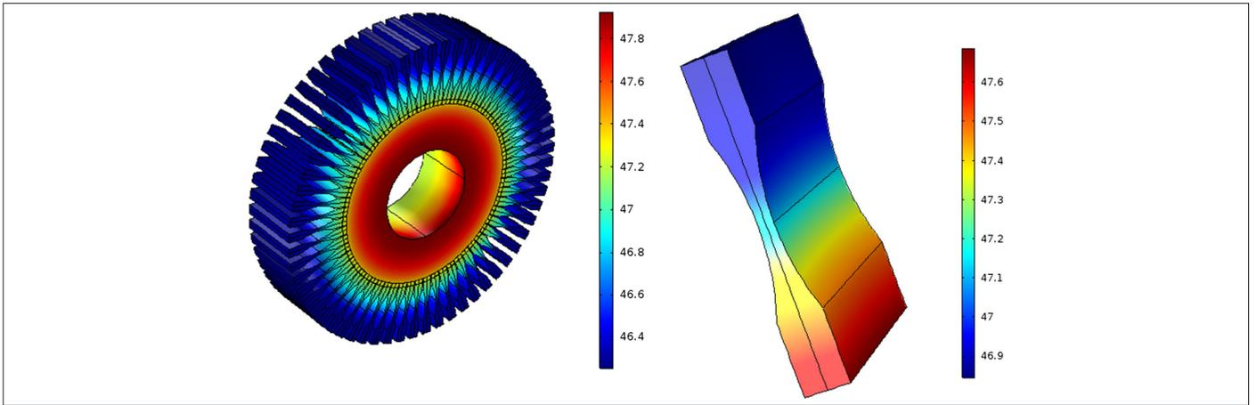
**Fig. 2.** Temperature distribution in proposed fin and heat sink.
