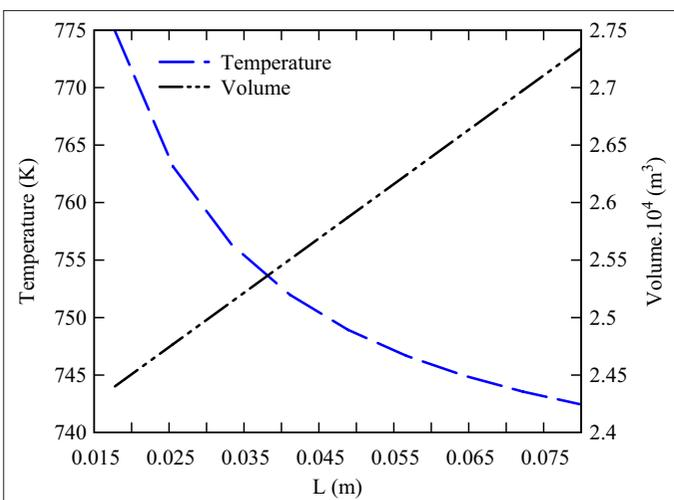
**Fig. 4.** Effect of fin's length on the mean temperature and volume.
